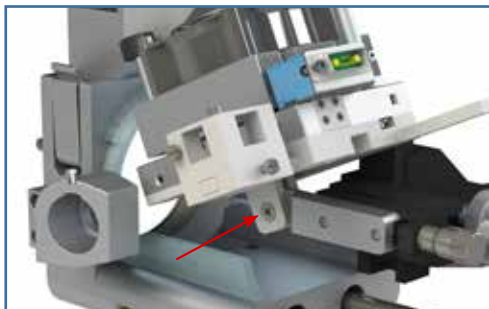
Fig. 8: Mounting the oven to the source
