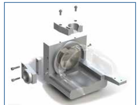
Fig. 5: Thermo Scientific ES071 source with mounting kit (exploded view)
