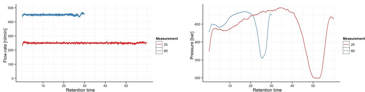
Figure 1: Flow-rate can be increased almost two-fold with an increase in temperature from 25°C to 60°C while keeping the pump pressure relatively stable.
