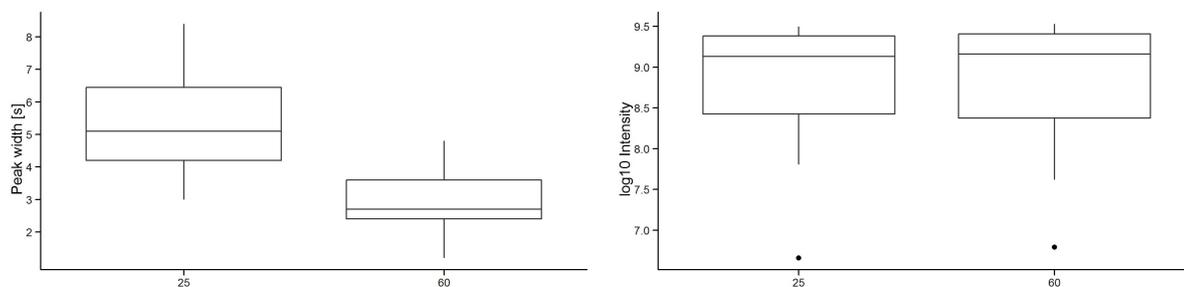
Figure 3: Reduced peak widths at a stable intensity per peak of a selection of tryptic BSA peptides.
