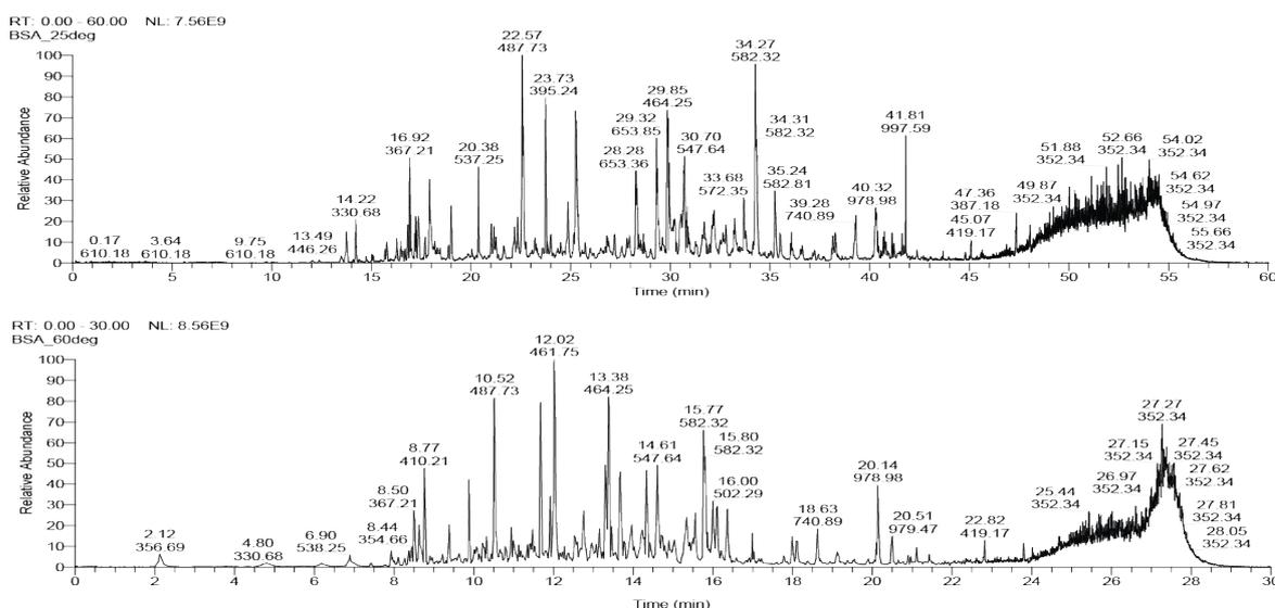
Figure 2: Comparison of base peak chromatograms, showing that separation is intact at the increased analysis speed.
